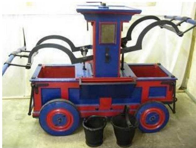
A double action water pump which might be similar to the one from Morgan's Brewery (with kind permission of Hungerford Virtual Museum)
